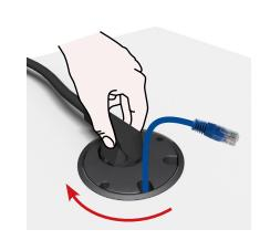
Rotate plug clockwise to reattach.
